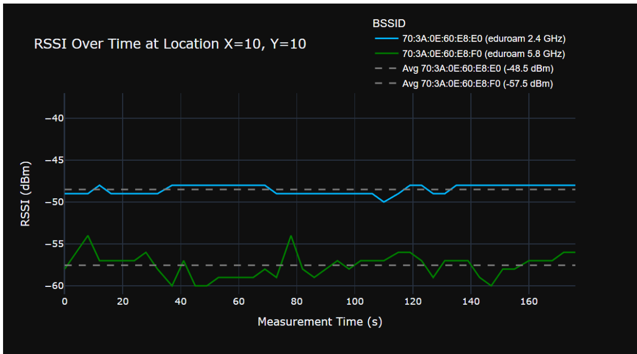
Figure 6: RSSI Over Time at Location X=10, Y=10.
